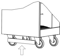
Lift weight straight up until hooks snap into place.
